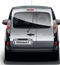
Glazed asymmetrical rear doors with wiper and demisting
